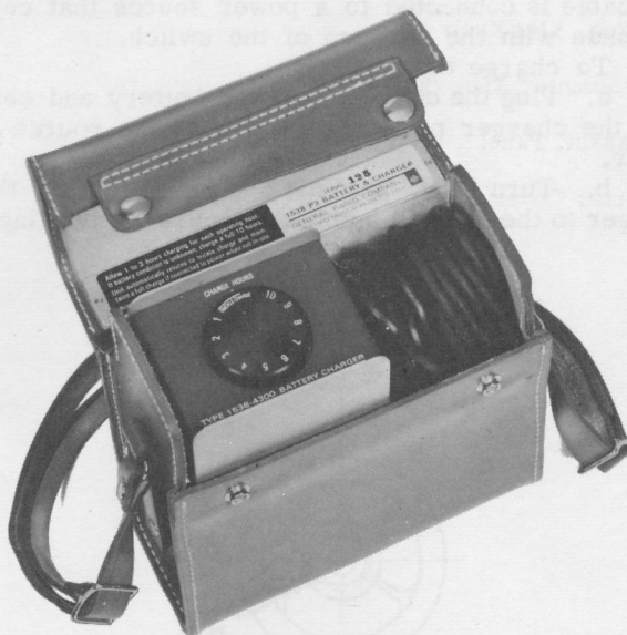
Figure. A-1. Battery and Charger.
